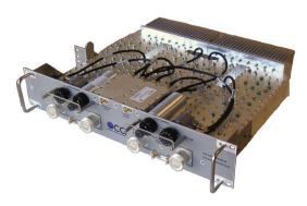
CCI's PCS Band DAS Interface Tray with "Independent Control" provides an integrated, convenient, and single connection point when using multiple base stations with a common DAS system. The unique architecture of the CCI DAS Interface Tray can simultaneously accommodate
