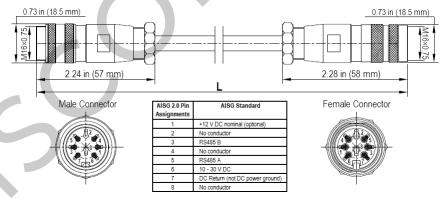
AISG-Male to AISG-Female Jumper Cable
