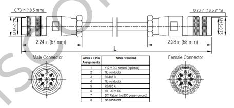
AISG-Male to AISG-Female Jumper Cable
