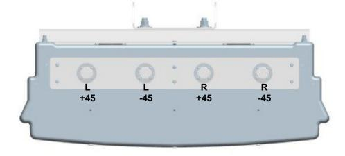
BSA-L65-17V010-62 Antenna Port Marking and Port Identification
