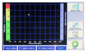
Figure 16 - PIM vs. Time Screen (Prior to Measurement)
