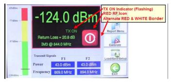
Figure 8 – PIM and Return Loss Screen with "TX ON"
