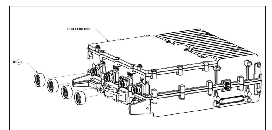
**Figure 2: Installation of Connector Boots**
