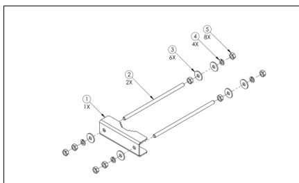
Fig. 7: Mast Bracket Clamp Only BOM
