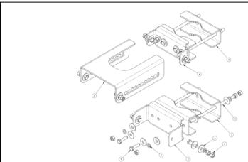
Fig. 1: Adjustable Mast Bracket BOM
