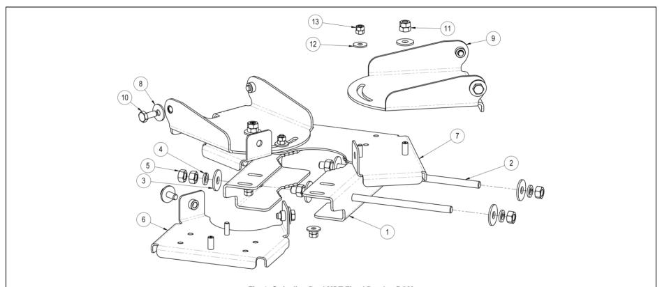
Fig. 1: Swiveling Dual MDT Fixed Bracket BOM
