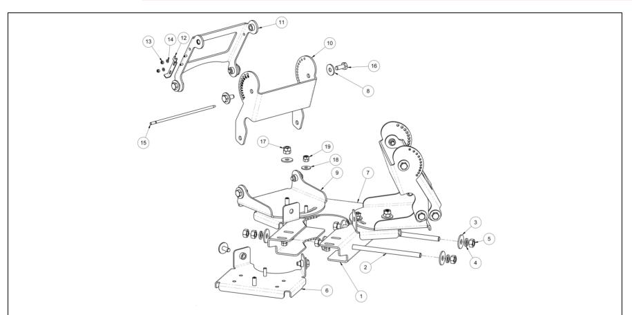
Fig. 2: Swiveling Dual MDT Adjustable Bracket BOM
