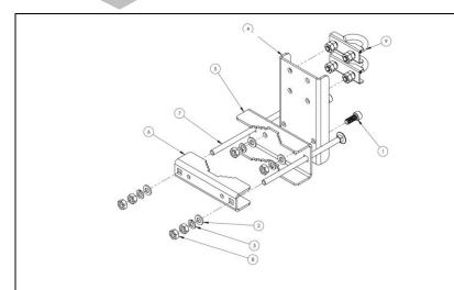
Fig. 1: MBC-09 Mast Bracket Clamp BOM
