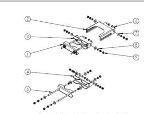
Fig. 1: Adjustable Mast Bracket BOM
