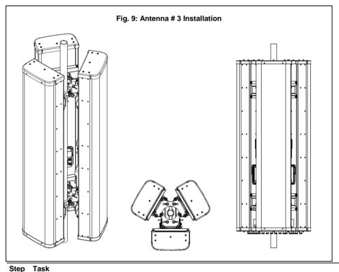
11 Install Antenna #3 on to Dual Hinge Brackets (Item 2) using M10 hardware (Items 8, 9, and 10) as shown in Fig. 9, and torque to 54 N·m (40 ft·lbs).
