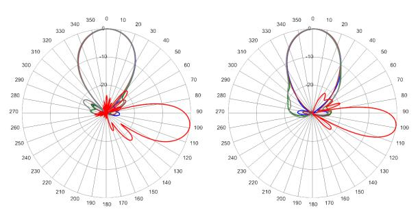
698 MHz Azimuth with Elevation 9°
