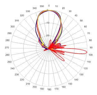
2340 MHz Azimuth with Elevation 6°
