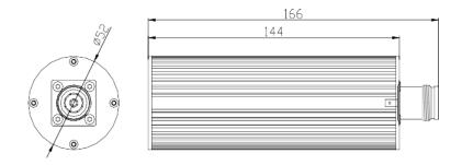
30 W Low PIM Termination Load with DIN Female Connector Outline Drawing
