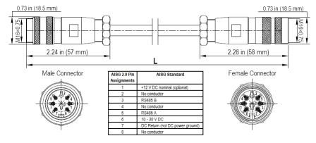
AISG-Male to AISG-Female Jumper Cable
