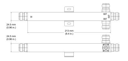
High Power 4-way Power Divider with N-type Female Connectors (PD-0727-4N) Outline Drawing
