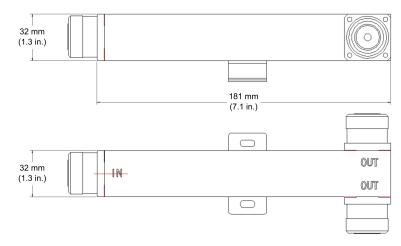
High Power 2-way Power Divider with DIN 7-16 Female Connectors (PD-0727-2D) Outline Drawing
