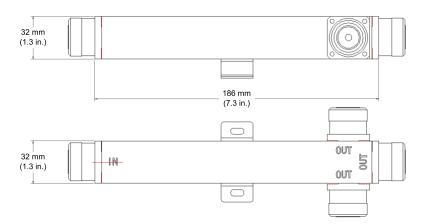
High Power 3-way Power Divider with DIN 7-16 Female Connectors (PD-0727-3D) Outline Drawing
