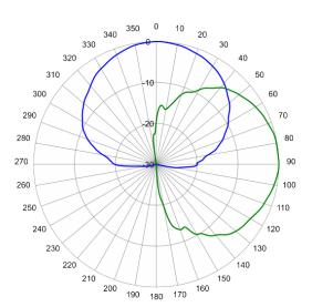
1780 MHz Azimuth with Elevation 0°
