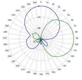
737 MHz Azimuth with Elevation 0°
