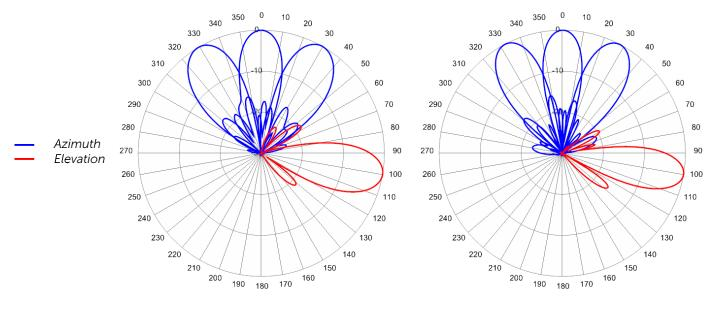
734 MHz Azimuth with Elevation 10°
