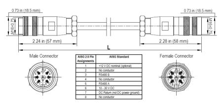
AISG-Male to AISG-Female Jumper Cable
