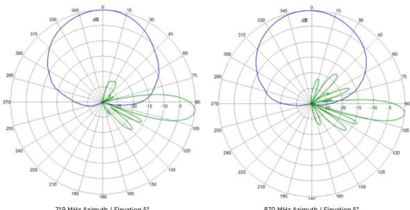
719 MHz Azimuth / Elevation 5°
