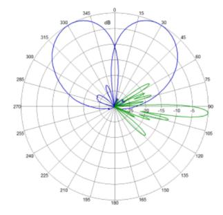
1920 MHz Azimuth / Elevation 4°
