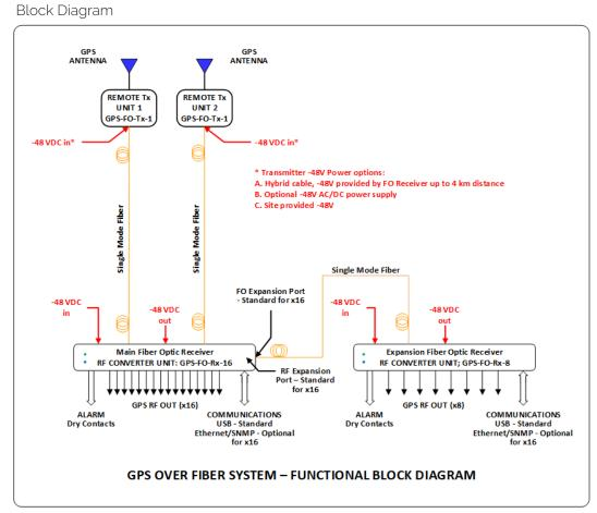
GPS Over Fiber System (GPS-FOS-T2R16-SA3P) Functional Block Diagram
