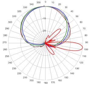
750 MHz Azimuth with Elevation 7°
