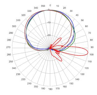
880 MHz Azimuth with Elevation 7°
