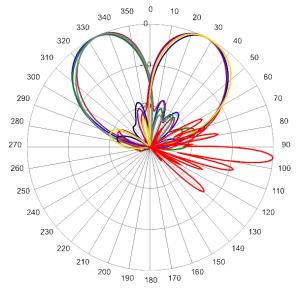
1920 MHz Azimuth with Elevation 5°
